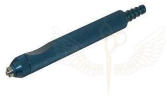
Product Description: Luer Lock Adjustable Handle ideal for rotating the Luer Lock flat to the thumb rest Handle diameter: 3/4" Overall length: 7.2" Body: Aluminum with type 2 blue anodized Male Luer Lock: Stainless Steel
